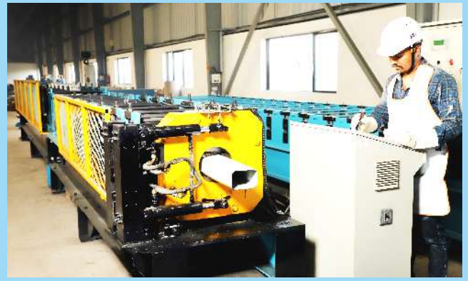
Downtake Pipe Profile Machine
